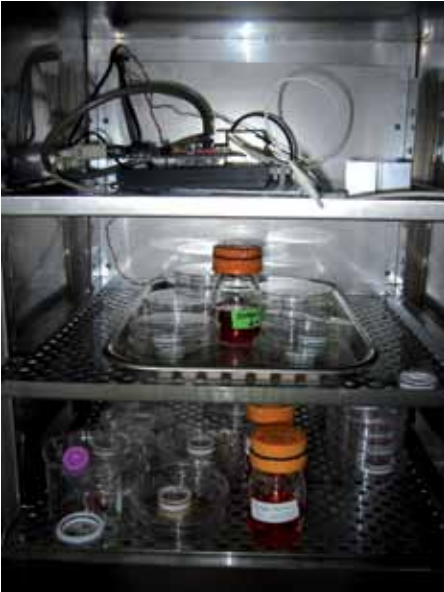
| Inkubator do hodowli tkanek: kultury neuronalne hodowane na szalkach MEA, roztwór pożywki w trakcie podgrzewania i stacja pomiarowa MEA na górnej półce, fot. dzięki uprzejmości artysty / Tissue culture incubator with Neural Cultures growing over MEA dishes, media solution heating up and MEA recording station on the top shelf. Photo taken at the Steve Potter Lab in Georgia Tech during a residency in 2006, photo courtesy of the artist
