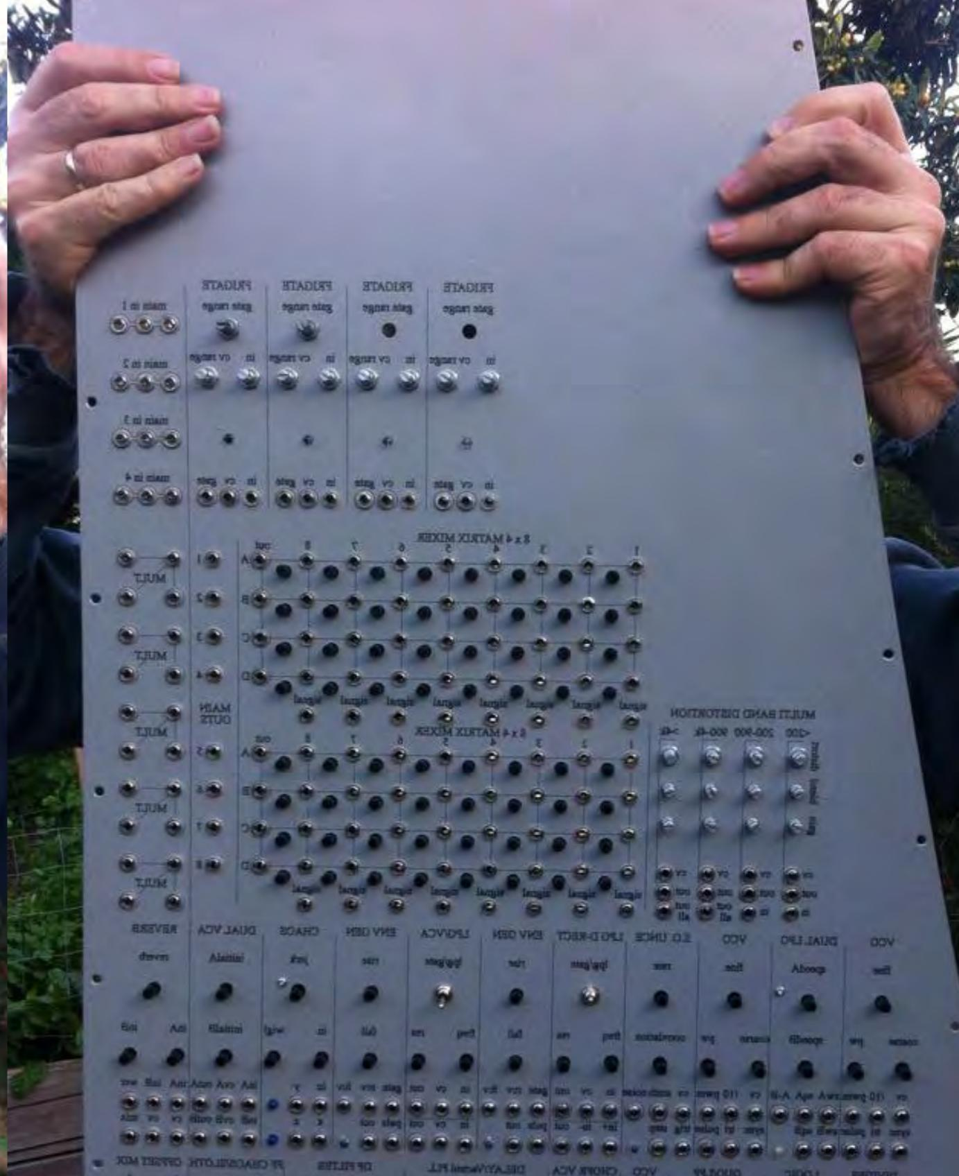
The neural networks were given a sound-producing body by connecting the MEA to a signal amplifier and a custom-built analogue synthesiser.
