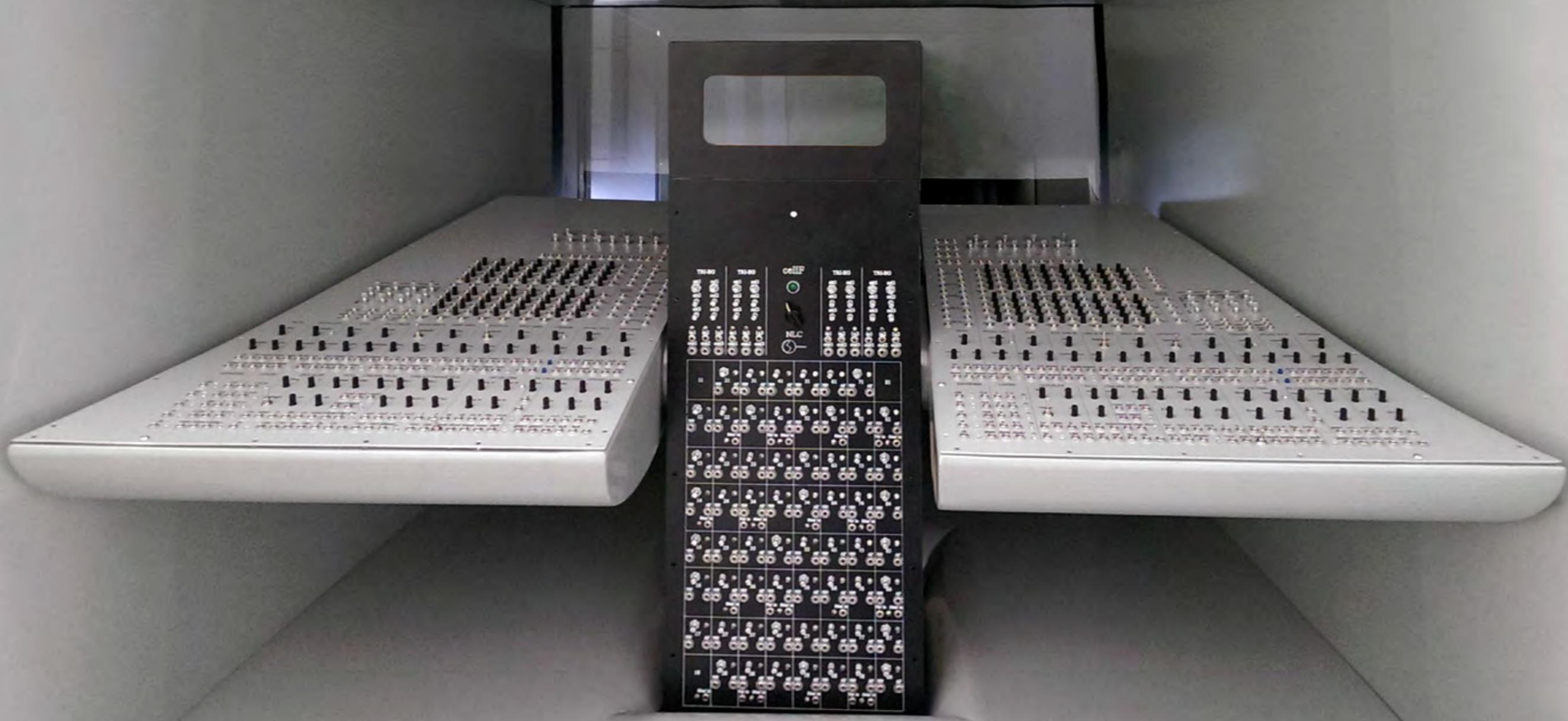
The neural interface is the heart of the entity. It enables 'communication' between the human performer and the neural network by controlling the input stimulations (human-generated sound) and the output signal (neural activity).
